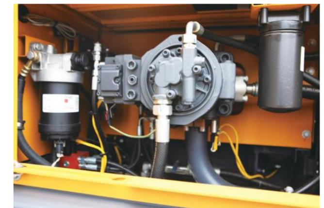
XE250U is suitable for medium volume earthwork working conditions. The larger flow of the main pump makes its hydraulic system very strong and can be matched with various operating tools. Finally, the XEICS intelligent control system, CAN bus, GPS controller and ECM engine management system are matched to improve data management efficiency and make operators more comfortable, safer and labor-saving. This excavator is mainly used in road and bridge, water conservancy, municipal construction, etc.
